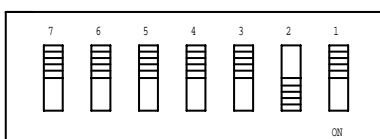
Figure 2-1, Switch S1 (Set to Logical Address 2)
